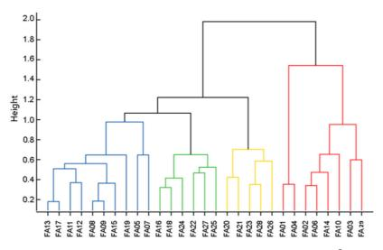
**Figure 5.** Cluster tree of the FA samples according to their content of Zn and Al<sup>0</sup>, the ANC, and the amount of FA produced in 2016. The y-axis shows the distances between the calculated values and hence is a mathematical value that expresses the dissimilarity.
