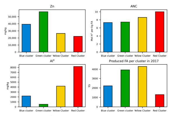
**Figure 6.** Average Zn and A<sup>10</sup> concentration as well as average produced FA per plant and the average ANC for each cluster.
