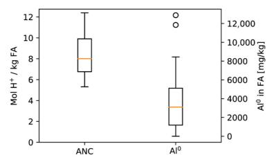
**Figure 4.** Boxplot of the acid neutralizing capacity (ANC) as amount mol  $H^+$  to reach pH 2 at a L/S ratio of 10 and  $Al^0$  in Swiss FA (n = 29).
