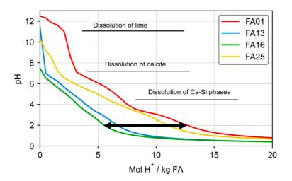
**Figure 3.** Titration curve of selected FA samples (LS 10). The main plateaus are marked with a black line. The black arrow illustrates the big difference of acid that is required to achieve pH 2.
