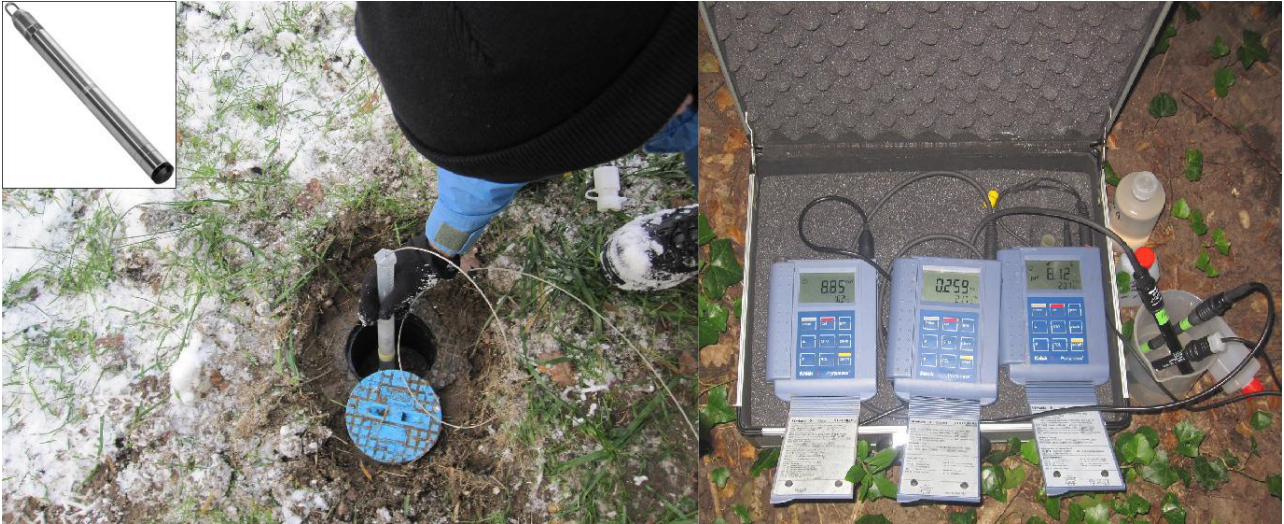
Logger DCX-22 AA and installation process and Knick Portames 911 devices for measuring pH , EC and DO
