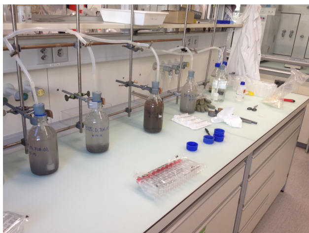
TVA CO 2 Eluate Test performed on the 4 MSWI Bottom ash. From left to right: MSWI_1, MSWI_4, MSWI_2 and MSWI_3.
