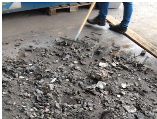
Bottom ash metals (>2 cm) manually separated from the MSWI_4 slags.
