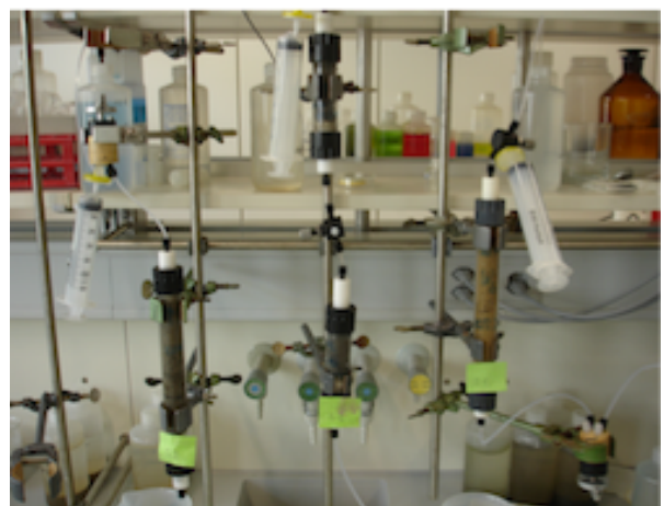
The three columns Left to right: Leaching experiment, uncontaminated top soil, uncontaminated bottom soil.
