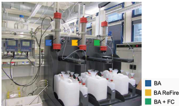
Column test experimental set up. The three columns are filled with Reference bottom ash (BA), ReFire bottom ash (BA ReFire) and a bottom ash-filter cake mixture (BA + FC).
